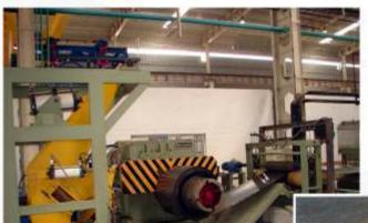
The ECL can have efficiency of up to 97.5% for the oil and in excess of 95% for the iron fines, depending of the quality of strip from the rolling operation. This is due to the combination of different processes to clean the strip: spray or dip cleaning, brushes, electro-cleaning section followed by a rinse built into different stages.
